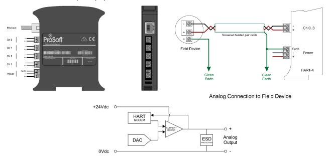
Analog Output Equivalent Circuit
