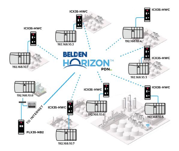
PDN is **simple** because to create the remote communications network, a user simply has to place the wired or wireless gateways in a project. The Belden Horizon<sup>TM</sup> platform is used to manage the network and the communication devices.
