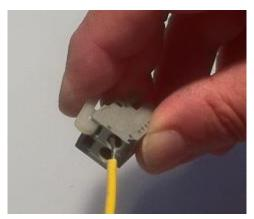
Press down on the installation tool to use it as a lever to open the connector's contacts to insert a wire. A properly-wired power connector is shown:
