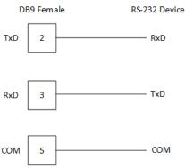
If hardware handshaking is required, the cable to connect to the port is as shown below:
