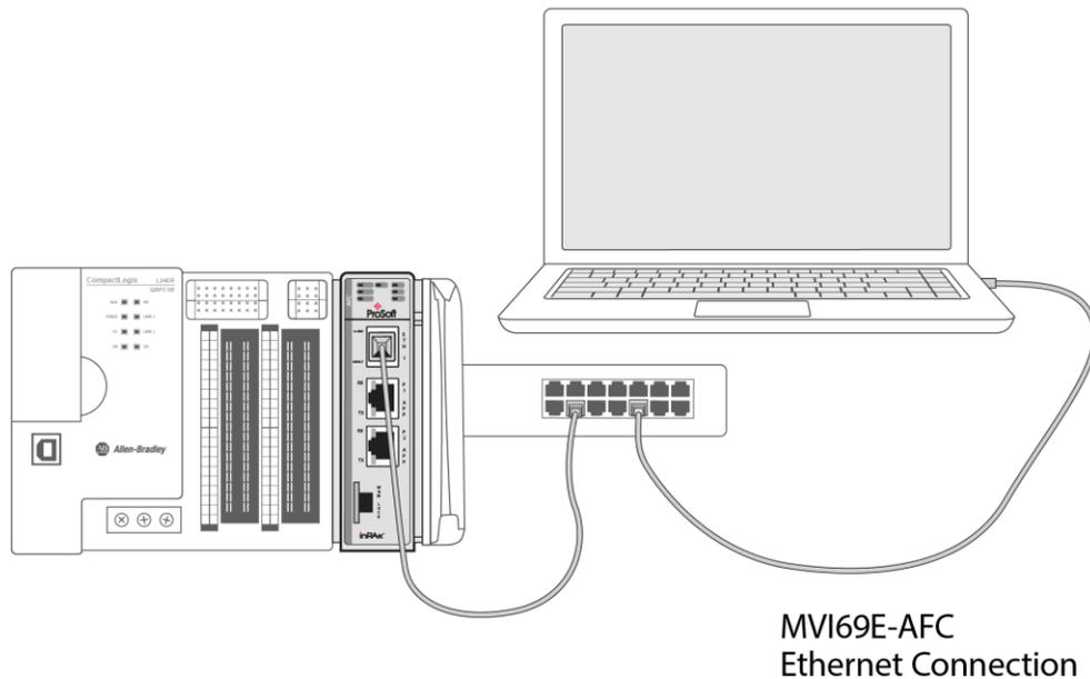
Connect the other end of the cable to the network. The PC running EAFC Manager must be on the same network.
