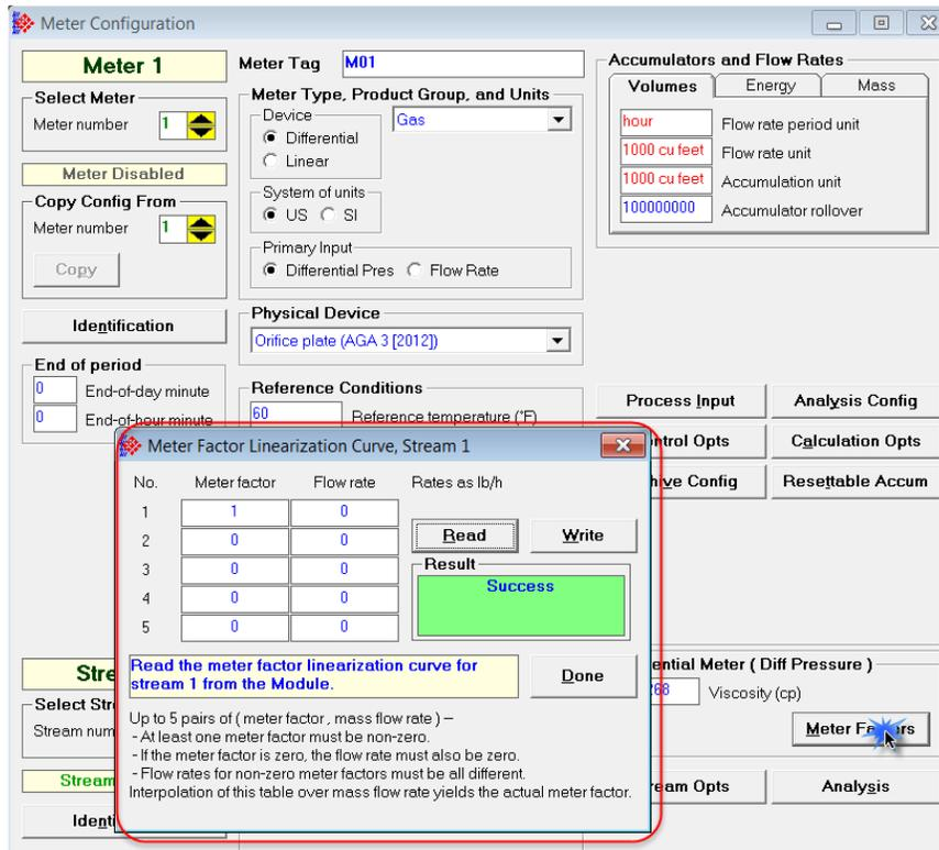
In the *Meter Factor Linearization Curve* dialog box, click the **READ** button to transfer the current Meter Factor Linearization configuration from the MVI69E-AFC to the local PC.
