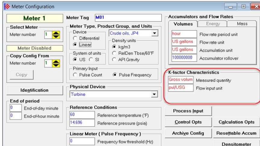
This area is visible when the meter type is Linear.
