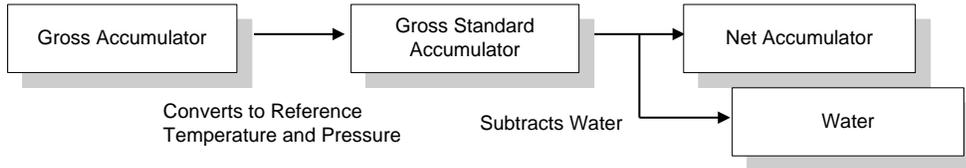
For liquid applications (Oil-Water Emulsion), the net accumulator is calculated as follows, using API ch 20.1:
