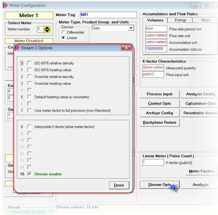
A meter always has one active stream which corresponds to the particular product that flows through the meter at that moment.
