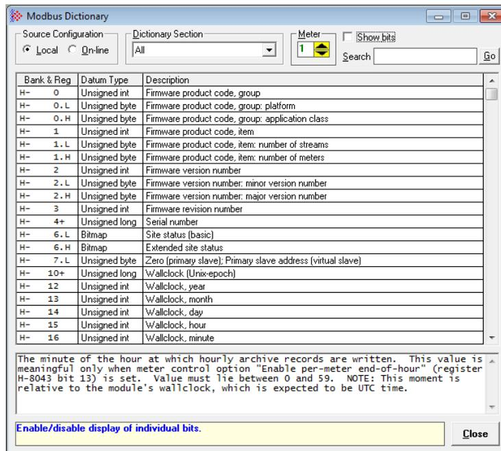
You can use the Modbus Dictionary locally or while EAFC manager is directly connected to the MVI69E-AFC module. From the *Source Configuration* section, select **LOCAL** if you are just running Modbus Dictionary locally or select **ON-LINE** if connected to a module.
