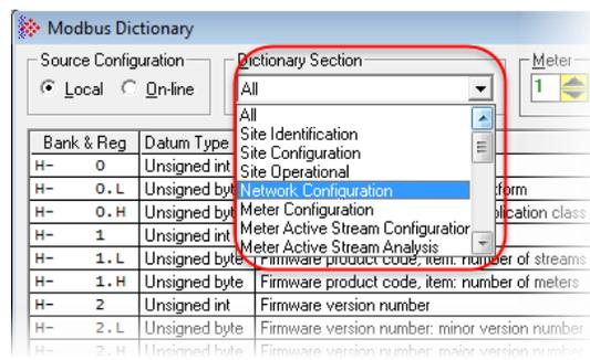
The *Meter* selection allows you to specify a specific meter in order to view only information pertaining to the selected meter.
