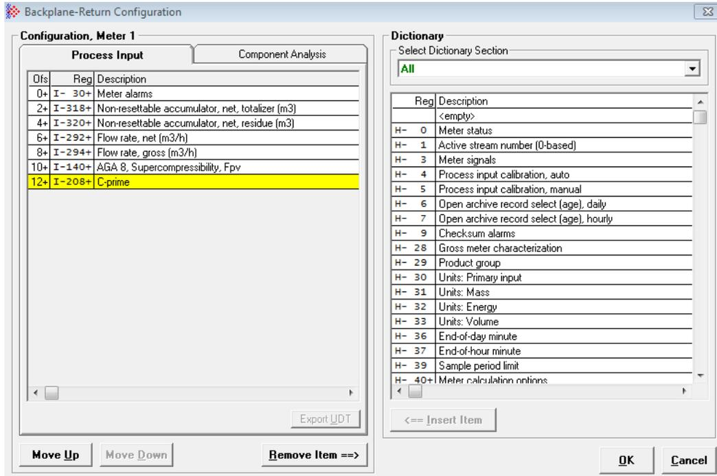
You can select desired values from the Modbus database which the module delivers to the PLC automatically and on a regular basis without having to create and issue a separate backplane transaction, such as Modbus Gateway in order to retrieve those values.
