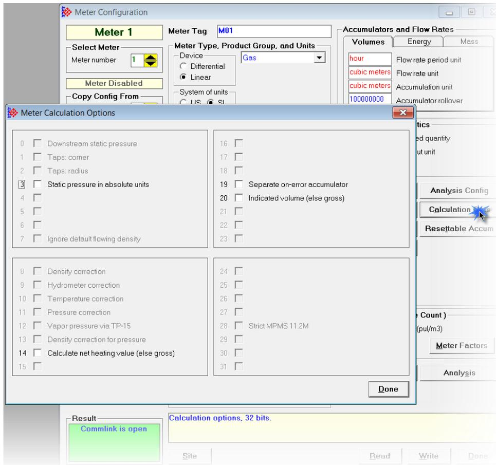
Options that do not apply to the current application are grayed out. See *Calculations Options* in the *MVI69E-AFC Reference Guide* for detailed information.
