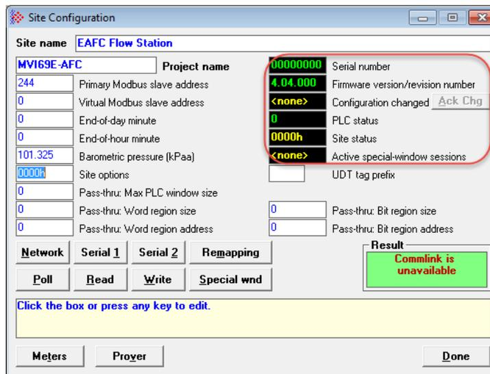
This section of the *Site Configuration* screen is used to provide Site status information. Site status features are discussed in the *MVI69E-AFC Reference Guide*.
