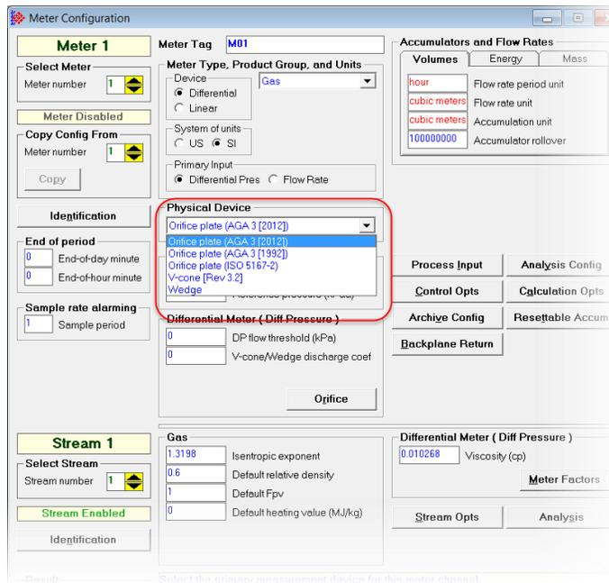
If you are using a differential gas type meter, measuring differential pressure, you have the option of selecting from the following standards:
