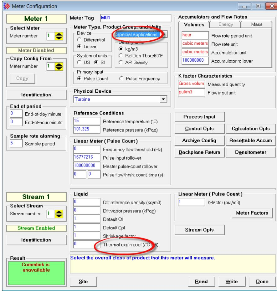
If the *Product Group* is set to **Oil-wtr emulsions (Crd)**, **Oil-wtr emulsions (NGL)**, all parameters are visible and **Water density @ 60°F (kg/m<sup>3</sup>)** is added. If the *Product Group* is set to **Produced/injected water**, the **Water Salinity (% mass)** parameter, along with the **Dflt reference density (°API)** are the only two parameters available.
