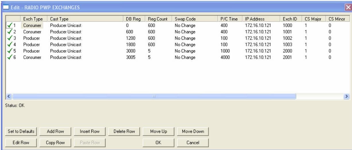
This is the area where you set up data exchange between the MCM modules. Communication is accomplished using Producer and Consumer commands. Using these commands, you specify the IP address of the receiving (Consumer) and sending (Producer) module as well as the database locations to produce data and receive data.
