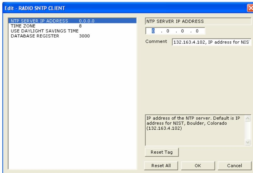
This section is used to synchronize the time using a centralized atomic clock. This feature is only usable if your modules are communicating through an access point such as a RadioLinx Industrial Hotspot. The values in this window should be left with the default values. As you select each parameter, the help window on the screen displays information to help you make your selections. The PWP Driver Manual describes each of these parameters.
