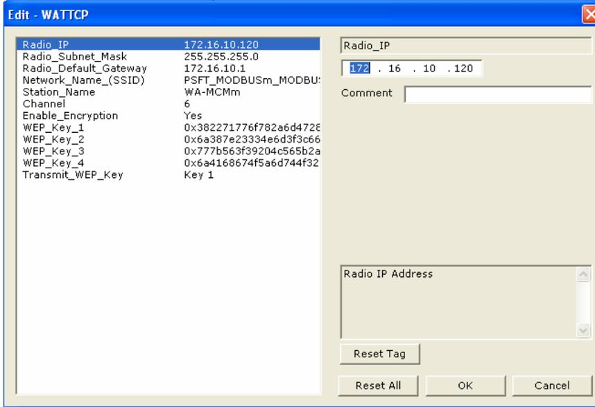
This section is identical for all 6201-WA-MCM modules shipped from the factory. The default Radio IP address is set to **172.16.10.120**. This IP address range is from 120 to 129.
