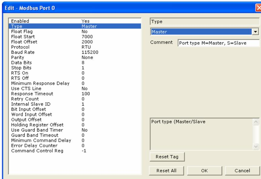
The "**Type**" parameter lets you specify whether the module is to be configured as a Master or a Slave. In this case, **Master** was selected since this is the MCM module connected to the remote slave. The remaining parameters are set to ensure that the MCM module can communicate with the slave. Refer to the MCM Driver Manual located on the ProLinx Solutions CD for detailed information on each of these parameters.
