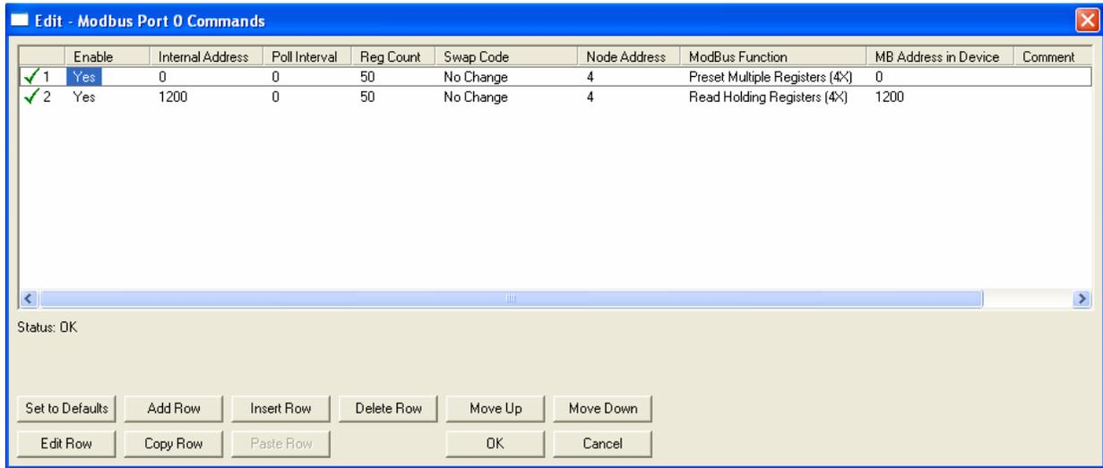
In the sample application, there is one slave device connected to the MCM Master module. This slave will read and write 50 words of data into the MCM master which in turn sends and receives this data between itself and the MCM slave. The command in this example shows how the data in the slave is passed through (and received from) the MCM master.
