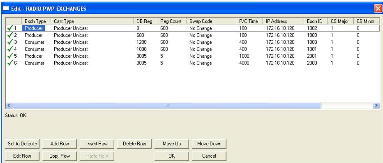
The commands in this section correspond to commands set up in the MCM master module. For example, the MCM master module has a Produce command to send data to the MCM slave. The MCM slave must have a corresponding Consume command to match up with the MCM master Produce command in order to accept the MCM master produced data.
