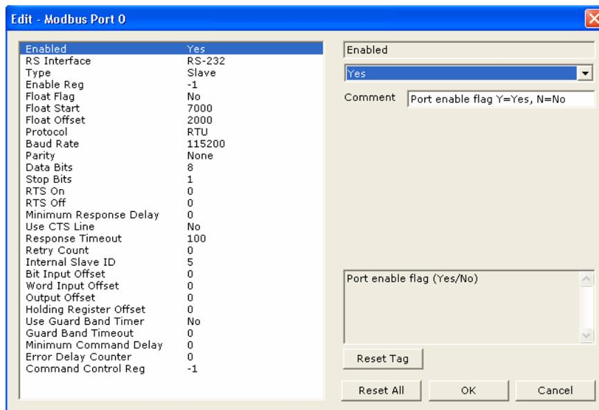
As with the 6201-WA-MCM Master, the 2nd module in the sample application must be configured as a slave in order to make the application work. This is done the same way as the master. Select the "**Type**" field and then select **Slave** from the drop-down list.
