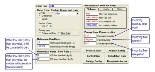
Choose Primary Input Characteristics according to the incoming flow rate delivered over the backplane.
