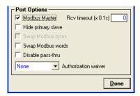
The Modbus Master command is generated from the processor using ladder logic (Modbus master block). After the Modbus Master transaction is completed the module is ready to receive another Modbus Master request from the ladder logic:
