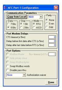
The Communication Parameters configure each port's communication settings. The default communication port configuration is 9600 baud rate, 8 data bits, 1 stop bit, RTU mode and no parity. Use these settings the first time you use AFC Manager on the port connected to the local PC.
