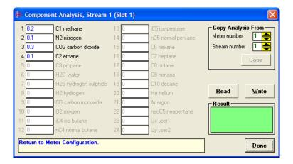
The module records events every time a molar concentration value changes. For applications that involve gas chromatograph devices, this feature might not be desirable because it is expected that the values should frequently change. You can disable this feature using AFC Manager (Meter Configuration / Control Options / Treat Analysis as Process Input).
