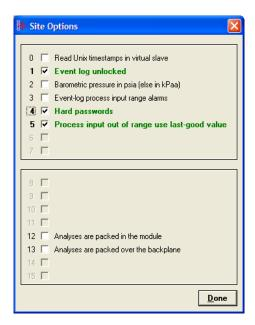
When this option is selected, any authorization granted using Hard Passwords times out after two minutes of inactivity, and the user will be required to re-enter the password to continue.
