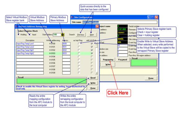
The values in the illustration above would configure the following indirect addressing remapping:
