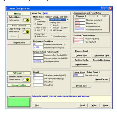
In the *Meter Configuration* dialog box above, Meter 1 is used in this example as the meter selected to be proved. It can be proved using any one of the four provers that the AFC supports. These provers are described in the *Prover Configuration* section. There is an Identification button which opens an editable options window, shown below. Text entered here appears on the proving report.
