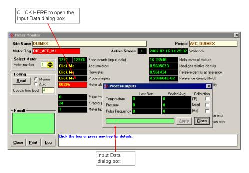
Using these data is particularly important when troubleshooting the meter run, since you can verify if the values transferred from the processor are correctly being received at the module.
