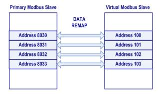
Because all registers in the example had the write enable bit set, all data copied to the Virtual Slave would also be written to the remapped Primary Slave. If a Modbus device writes a value to address 100 in the Virtual Slave, that value would also be written to address 8030 in the Primary Slave. If it reads the current value on the Virtual Slave address 102, it would be the same value in Primary Slave address 8032.
