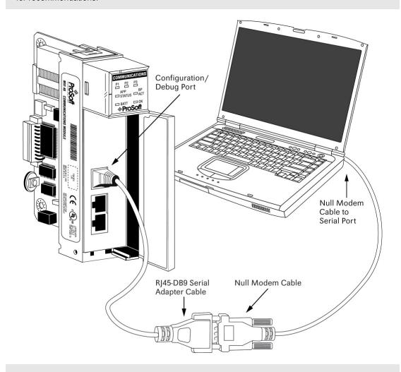
**Note:** The illustration above shows an MVI46-AFC. The connection process is similar for all MVI-AFC and PTQ-AFC models.
