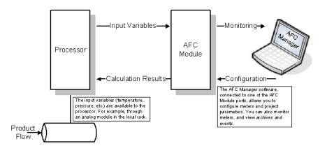
You can configure each meter in the local computer (saving the configuration as a .AFC file) and then download the file to the module. Later, you can adjust specific meter configuration parameters without downloading the entire project; this is accomplished using the Write button in the Meter Configuration dialog box. You can also transfer the current configuration from the module to the local computer by uploading the current configuration.
