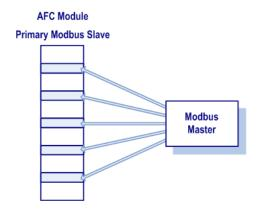
However, using the Virtual Modbus Slave optimizes the polling of data because the registers can be remapped in any order using the AFC Manager (Site Configuration window). The following illustration shows how the orifice diameter registers could be remapped to the Virtual Slave starting at address Vh00100:
