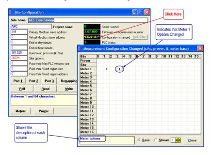
After you have verified the Measurement Configuration Changes, click the Ack Chg button on the Site Configuration dialog box to clear the bits in order to keep track of future changes.
