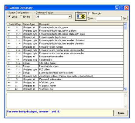
The information in this dialog box is "read-only", meaning that you cannot edit values here. To configure data remapping, refer to Primary & Virtual Modbus Slave Configuration (page 36).
