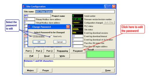
The module supports two passwords: Write-Enable and Read-Only. Each password is enabled when you write a non-zero value to the corresponding register.
