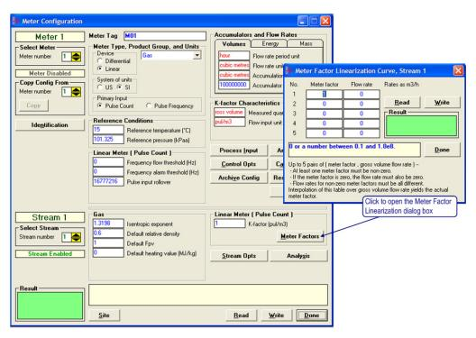
Click the Meter Factor Curve **Read** button to transfer the current Meter Factor Linearization configuration from the AFC module to the local PC
