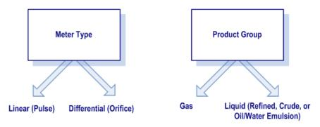
**Note:** The meter channel must disabled in order to change its meter type and product group.
