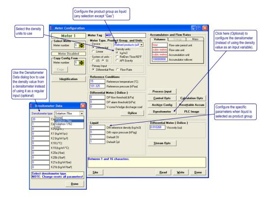
This area is visible when the product group is set to a liquid group. Enter the values for Default Reference Density, Vapor Pressure, Default Ctl and Default Cpl. The following parameters are required for the calculations.
