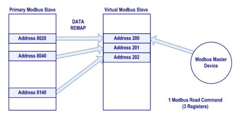
When the registers are remapped into a contiguous group in the Virtual Slave, the master can use a single Modbus command to poll the registers. This results in better system performance, because the number of commands is reduced.
