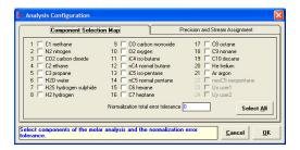
Select (check) the components to be analyzed, enter the Normalization total error tolerance value, and then click Done.
