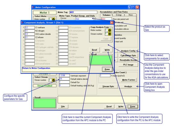
The following parameters are required for the calculations.
