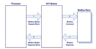
The following Modbus functions are supported for Modbus Master operation:
