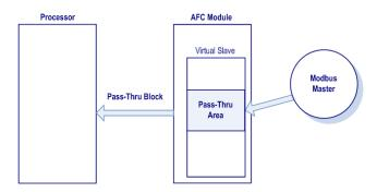
**Important:** You must enable the virtual slave by configuring a Modbus address greater than 0 (**Project / Site Configuration**).
