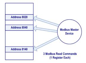
For this application, the master reads three MODBUS registers: 8020, 8040 and 8140. As these registers are not contiguous, the master uses three Modbus commands to poll all the registers.
