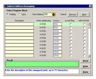
The following table shows how the addresses would be remapped between both slaves:
