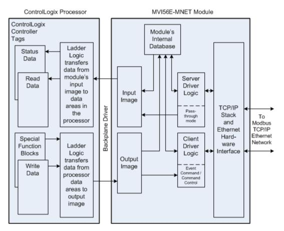
All data transferred between the module and the processor over the backplane is through the input and output images. Ladder logic must be written in the ControlLogix processor to interface the input and output image data with data contained in the controller tags. All data used by the module is stored in its internal database. This database is defined as a virtual Modbus data table with addresses from 0 (40001 Modbus) to 4999 (45000 Modbus).
