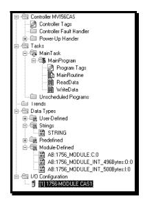
The next step in the module's setup is to define the User Defined Data Types to be used with the module. Copy these data types from the example ladder logic if you are not using the example. They will be defined if you are starting from the example ladder logic. The Controller Organization window should display the User Defined Data Types shown below:
