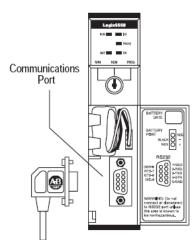
8 Connect the straight connector end of the cable to the serial port on your computer.
