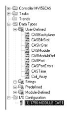
The next step in module setup is to define the data to be used to interface with the module and the ladder logic. Open the Controller Tags Edit Tags dialog box and enter the values shown in the following example. The MVI56-CAS module is defined in the example as CAS1. You can set the tag name to any valid tag name you desire. If you are using the example ladder logic, this step has already been performed.
