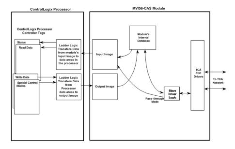
As shown in the diagram above, all data transferred between the module and the processor over the backplane is through the input and output images. Ladder logic must be written in the ControlLogix processor to interface the input and output image data with data defined in the Controller Tags. All data used by the module is stored in its internal database. This database is defined as a data table with addresses from 0 to 6999. The following illustration shows the layout of the database:
