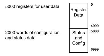
Data contained in this database is paged through the input and output images by coordination of the ControlLogix ladder logic and the MVI56-CAS module's program. Up to 248 words of data can be transferred from the module to the processor at a time. Up to 247 words of data can be transferred from the processor to the module. Each image has a defined structure depending on the data content and the function of the data transfer as defined below.
