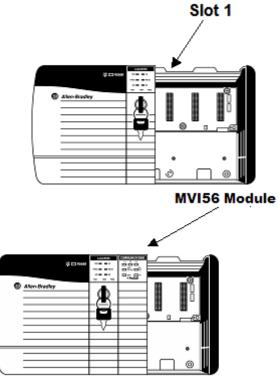
5 With a firm but steady push, snap the module into place.
