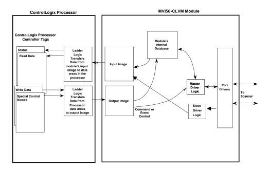
As shown in the diagram above, all data transferred between the module and the processor over the backplane is through the input and output images. Ladder logic must be written in the ControlLogix processor to interface the input and output image data with data defined in the Controller Tags. All data used by the module is stored in its internal database. This database is defined as a virtual data table with addresses from 0 to 2999. The following illustration shows the layout of the database:
