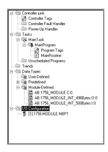
The next step in the module's setup is to define the User Defined Data Types to be used with the module. Copy these data types from the example ladder logic if you are not using the example. They are defined if you are starting from the example ladder logic. The Controller Organization window should display the User Defined Data Types shown in the following example:
