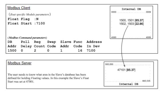
**Float Flag: "N"** tells the client to ignore the floating values and treat each register data as a data point composed of 1 word, 2 bytes or 16 bits.
