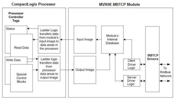
All data transferred between the module and the processor over the backplane is through the input and output images. Ladder logic in the CompactLogix processor interfaces the input and output image data with data defined in the Controller Tags. All data used by the module is stored in its internal database. This database is defined as virtual MBTCP data tables with addresses from 0 to the maximum number of points for each data type.
