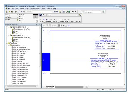
The setup procedure is now complete. Save the project. It is ready to download to the CompactLogix processor.
