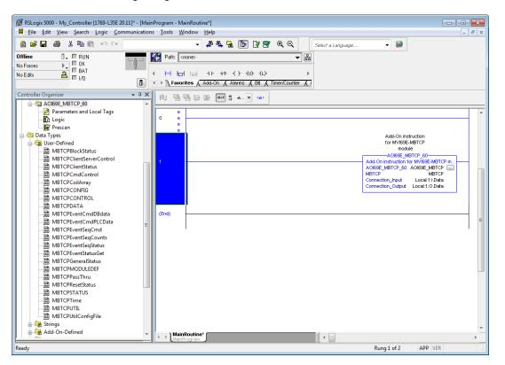
The procedure has also imported new user-defined data types, data objects and the Add-On instruction to be used in the project with the MVI69E-MBTCP module.
