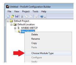
4 In the *Choose Module Type* dialog box, select **MVI69E** in the **PRODUCT LINE FILTER** area, and then select **MVI69E-MBTCP** as the **MODULE TYPE**. Click **OK**.
