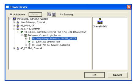
**Note:** DF1 serial download via CIPConnect is not supported. Only use Ethernet or EtherNet/IP drivers via RSWho.
