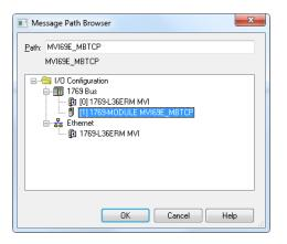
4 The module name is displayed in the *Path* field. Click **OK** to confirm the route configuration.
