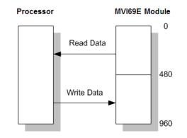
Database address 0 to 479 is continuously transferred from the module to the processor. Database address 480 to 959 is continuously transferred from the processor to the module.
