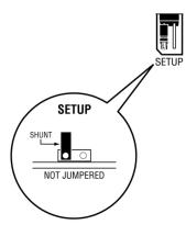
**Note:** If you are installing the module in a remote rack, you may prefer to leave the Setup pins jumpered. That way, you can update the module's firmware without requiring physical access to the module.
