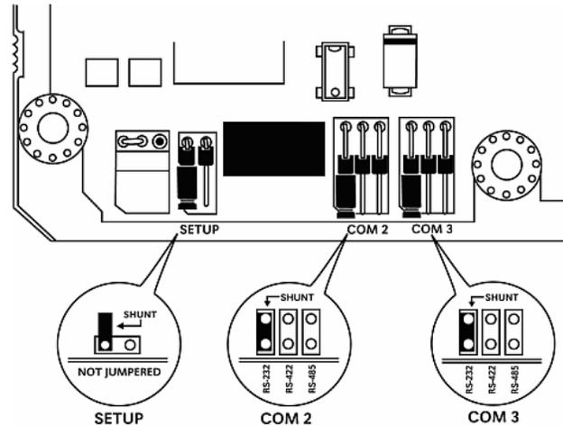
The Setup Jumper acts as "write protection" for the module's flash memory. In "write protected" mode, the Setup pins are not connected, and the module's firmware cannot be overwritten. Do not jumper the Setup pins together unless you are directed to do so by ProSoft Technical Support.
