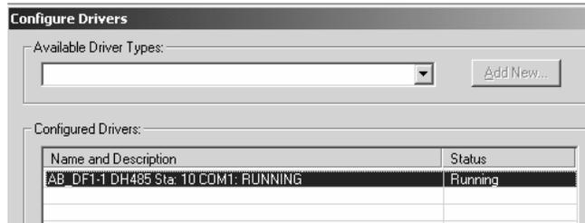
If you see the status as running, you will not be able to use this com port for anything other than communication to the processor. To stop the driver press the "Stop" on the side of the window:
