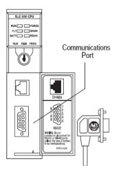
**2** Connect the straight connector end of the cable to the serial port on your computer.
