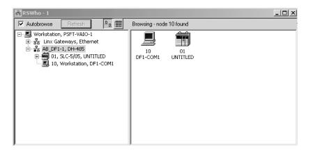
3 Notice how the DF1 driver is opened, and the driver is looking for a processor on node 1. If the network is being browsed, then you will not be able to stop this driver. To stop the driver your RSWho screen should look like this:
