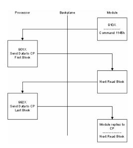
Block ID for the transfer of data from the processor to the module to be sent out the serial port
