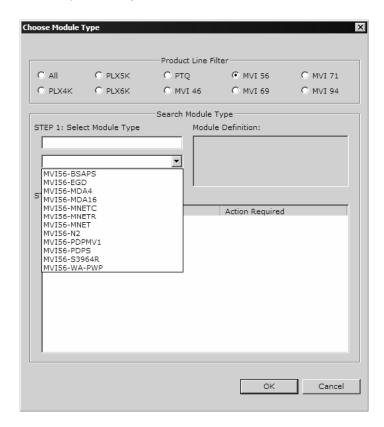
In the Product Line Filter area of the dialog box, select MVI56. In the Select Module Type dropdown list, select MVI56-S3964R, and then click OK to save your settings and return to the ProSoft Configuration Builder window.
