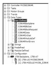
After you have defined the User Defined Data Types, the next step is to define the data to be used to interface with the module and the ladder logic. Open the Controller Tags Edit Tags dialog box and enter the values shown in the following example. The MVI56-S3964R module is defined in the example as S3964R. You can set the tag name to any valid tag name you desire. If you are using the example ladder logic, this step has already been performed.
