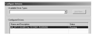
If you see the status as running, you will not be able to use this com port for anything other than communication to the processor. To stop the driver press the "Stop" on the side of the window:
