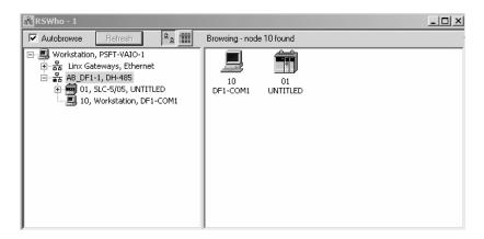
Notice how the DF1 driver is opened, and the driver is looking for a processor on node 1. If the network is being browsed, then you will not be able to stop this driver. To stop the driver your RSWho screen should look like this:
