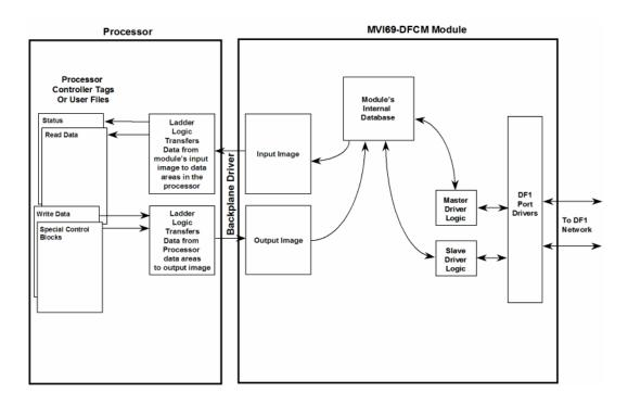
The following illustration shows the data transfer method used to move data between the CompactLogix or MicroLogix processor, the MVI69-DFCM module and the DFCM network.
