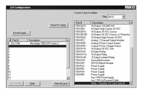
3 On the I/O Configuration dialog box, select "Other - Requires I/O Card Type ID" at the bottom of the list in the right pane, and then double-click to open the Module dialog box.
