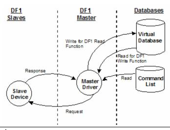
Each command issued from the DF1 master contains a field that indicates the location in the virtual database to be associated with the command. Care must be taken when designing a system to be sure the read and write data regions for the database do not overlap for a single device. The read area of one device can overlap the write section of another device to transfer the data from one slave device to another.
