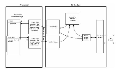
As shown in the diagram, all data transferred between the module and the processor over the backplane is through the input and output images. Ladder logic must be written in the CompactLogix or MicroLogix processor to interface the input and output image data with data defined in the controller tags. All data used by the module is stored in its internal database.
