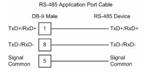
Note: Terminating resistors are generally not required on the RS-485 network, unless you are experiencing communication problems that can be attributed to signal echoes or reflections. In this case, install a 120 ohm terminating resistor on the RS-485 line.
