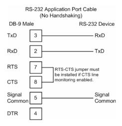
Note: If the port is configured with the "Use CTS Line" set to 'Y', then a jumper is required between the RTS and the CTS line on the module connection.
