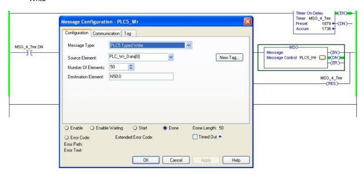
This sample assumes that a 1756-ENBT/ EN2T/EN3T module is in Slot 1 which is the second parameter listed in the path below. The IP Address is the IP Address of the AN-X2 Gateway.
