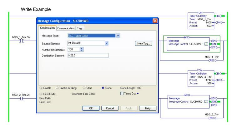
This sample assumes that a 1756-ENBT/ EN2T/EN3T module is in Slot 1 which is the second parameter listed in the path below. The IP Address is the IP Address of the AN-X2 Gateway.
