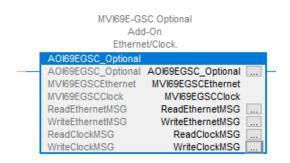
When importing this rung into a program, you may need to change the "Communication Path" of each of the message instructions to match the slot of the module in your program. This can be done by selecting the MSG tag and going to the Communication tab as shown below:
