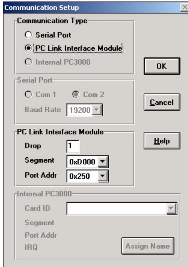
3. Set the *Communications Type* to PC Link Interface Module.
