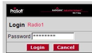
**Important:** The radio configuration is protected by a login password. The default password for the radio is "password" (lower case, no quotes). To prevent unauthorized access to the radio configuration, you should change the password when you have finished the initial configuration.
