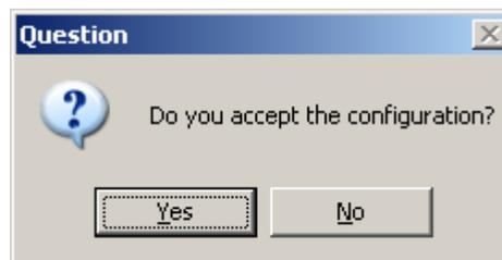
If accepted, the *network scan* window will close and the *PROFIBUS Master Configuration* window will be populated with the slaves that were found during the network scan.
