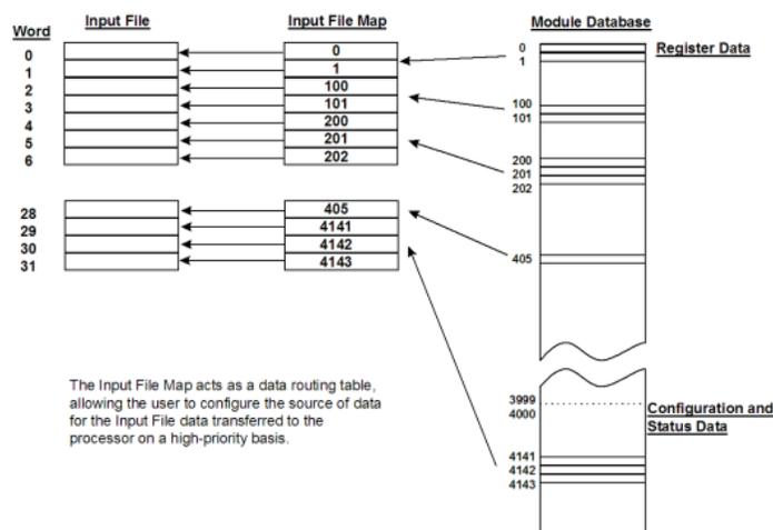
Each time the module enters a new read block into the input image it uses this Input File Map to select data out of the module's database and places it in the input image. Any data in the module's database can be assigned to the high-speed Input File data using this map.
