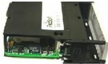
Do not change the position of the Setup jumper unless instructed to do so by ProSoft Technical Support.
