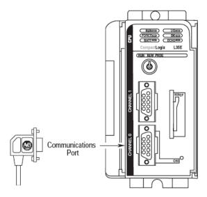
**2** Connect the straight connector end of the cable to the serial port on your computer.
