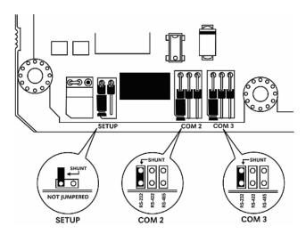
The Setup Jumper acts as "write protection" for the module's flash memory. In "write protected" mode, the Setup pins are not connected, and the module's firmware cannot be overwritten. Do not jumper the Setup pins together unless you are directed to do so by ProSoft Technical Support.
