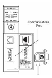
**2** Connect the straight connector end of the cable to the serial port on your computer.
