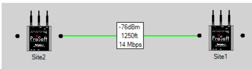
As you can see, the transmission speed of the wireless connection is dependent on the strength of the signal, and declines as the distance between the radios increases. In an industrial application, this can lead to poor performance or even lost connections.
