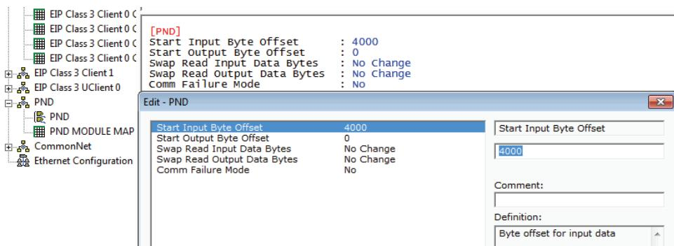
The default addresses will be used in this document. The PROFINET Input data will start on byte 4000 (Integer register 2000), and PROFINET Output data will start on byte/register 0.
