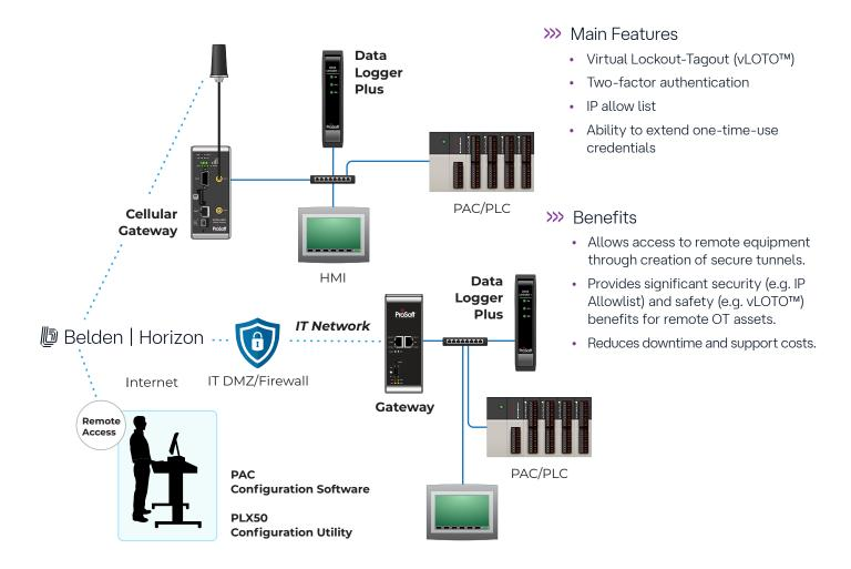
This type of remote connection is for a specific purpose. Examples include checking status, changing PAC software or upgrading firmware. The user will disconnect once the action has been completed.
