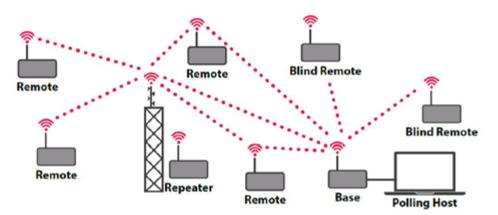
A traditional SCADA system architecture based on licensed or unlicensed radio communications to remote sites.
