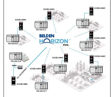
This type of remote connection is used to connect geographically dispersed locations for a SCADA type network, like monitoring a municipal water utility or a gas distribution network. PDN is like being plugged into a local switch.
