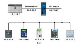
Other protocol solutions are available, including modules supporting IEC-60870-5-101/103/104, Modbus, PROFIBUS, and PROFINET.
