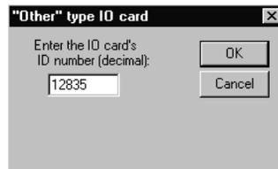
Enter the module I/O card ID number as 12835, and then click OK. Double-click the mouse on the module just added to the rack. Fill in the dialog box as shown:
