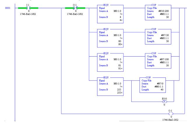
Blocks 80 and 81 handle the Modbus command data. Only two blocks (10 commands) are used here, but the command blocks could potentially reach 99 if 100 commands are used.
