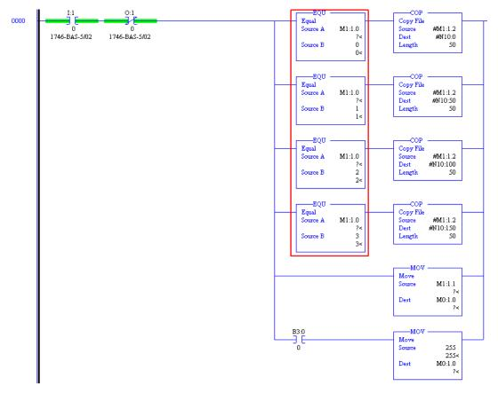
N7:24 in this configuration is particularly useful in a Modbus master application, that determines where the in the MCM memory the module stores a status word for each Modbus command. In this example, N7:24 is 150 which would correspond to block ID 3 in the input rung of the MCM logic. Looking at the above rung, we can see that the Modbus command status data will be stored starting at N10:150.
