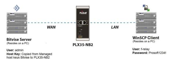
1 From the WinSCP Client, open a SFTP session to PLX35-NB2 and transfer few files to the *Upload* folder on PLX35-NB2 SD card:
