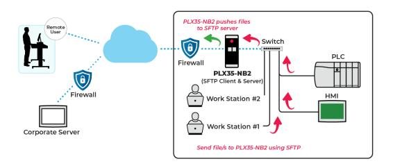
The *File Relay* tab allows you to use the SD card port on the device as a temporary storage medium for large files that can be automatically transferred to a remote location. Files can be copied to the PLX35-NB2 SD card from an FTP/SFTP Client. The files can then be transferred to a remote FTP/SFTP Server, or via Belden Horizon.
