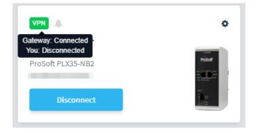
This example shows a connection between the gateway and the VPN server. However, it shows the user as "Disconnected". In this case, Belden Horizon may be waiting for the user to provide a user name in order to connect to the VPN.
