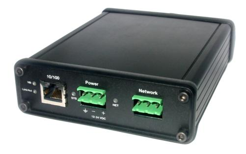
The RIO-HMI communications module is used to connect HMI, SCADA, or MES systems to data on an Allen-Bradley Remote I/O network. Typical applications for this module include replacing obsolete HMIs with built-in Remote I/O cards with newer HMI terminals that connect to an EtherNet IP network such as a Panelview Plus 6. For applications where multiple HMI terminals exist on a single Remote I/O network a single AN-X2 gateway can be used to provide data to these HMI terminals.
