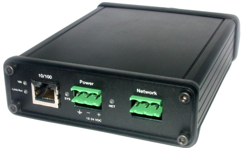
The RIO-HMI communications module is used to connect HMI, SCADA, or MES systems to data on an Allen-Bradley Remote I/O network. Typical applications for this module include replacing obsolete HMIs with built-in Remote I/O cards with newer HMI terminals that connect to an EtherNet IP network such as a Panelview Plus 6. For applications where multiple HMI terminals exist on a single Remote I/O network a single AN-X2 gateway can be used to provide data to these HMI terminals.
