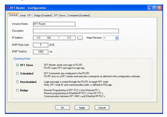
2. Go to the DF1 Slave tab, then configure the path to the logix controller in Logix Controller Mapping and assign a name to this map. In Logix Tag Mapping configure a DF1 Node and Data File that will be emulated in DF1 side, then select the Logix PLC in Target Name and finally write or browse the array tag placed in Controller tags in Target Tag field.
