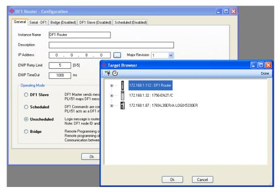
7. Go to the **Serial – DF1** tab and configure the basic serial communication parameter to match with PLC5 Chanel 0 configuration (see section III in this document).
