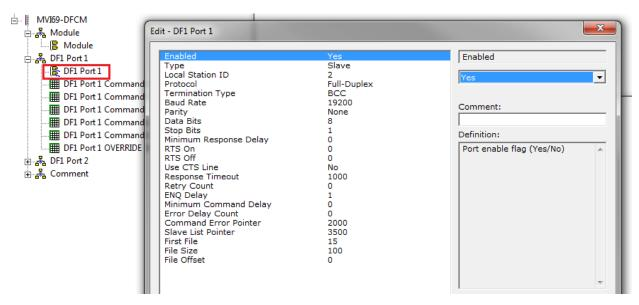
The MVI69-DFCM module is configured under these parameters:
