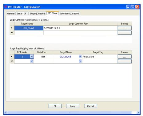
Note that in both cases the modules are mapping the Data File N15, so the PLC5 is going to write to or read from it.
