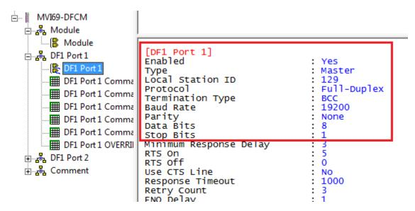
The MVI69-DFCM module is configured under these parameters:
