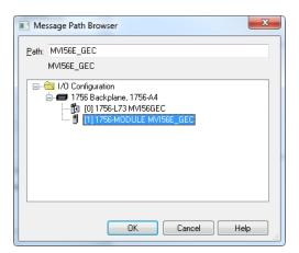
**4** The module name is now displayed in the *Path* field. Click **OK** to confirm the route configuration.
