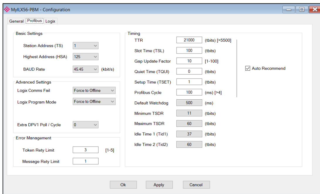
Figure 3.13 – ILX56-PBM PROFIBUS configuration – Master Mode
