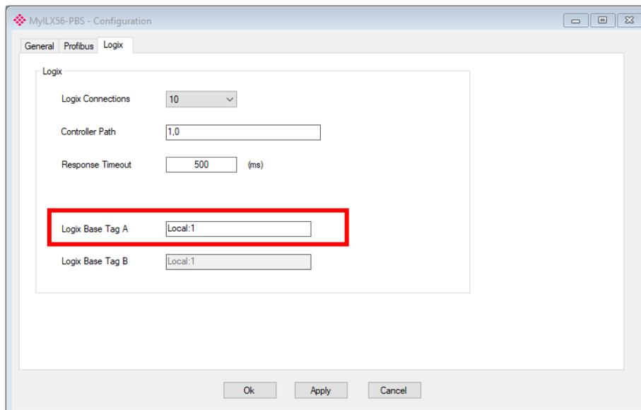
Figure 3.34 – Logix Base tag assignment in PLX50CU
