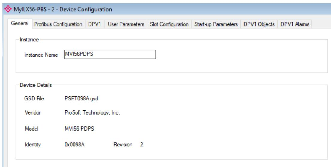
Figure 3.12 – Device General configuration parameters (legacy device)
