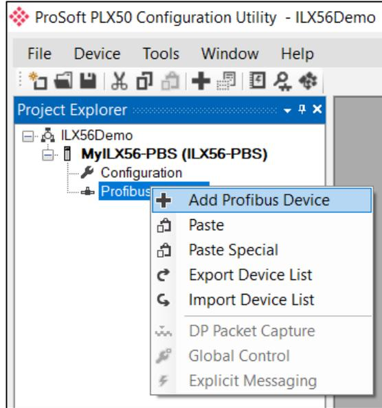
Figure 3.9 – Adding a PROFIBUS Field Device
