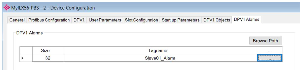
Figure 3.24 – Device DPV1 Alarms configuration parameters (Logix)
