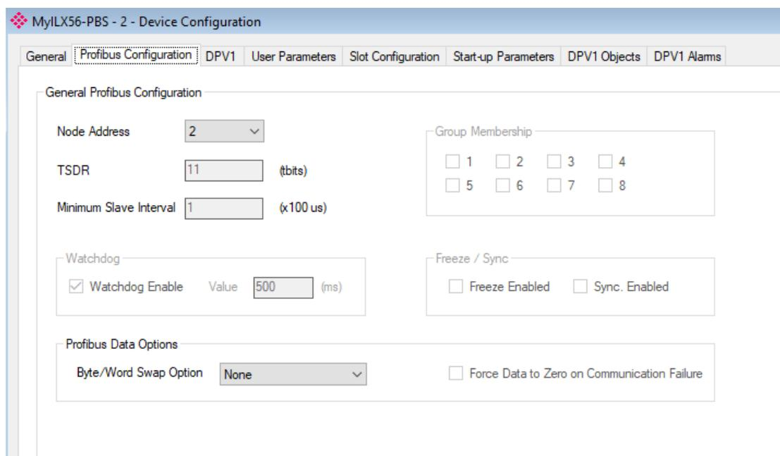
Figure 3.14 – Device PROFIBUS configuration parameters (legacy device)
