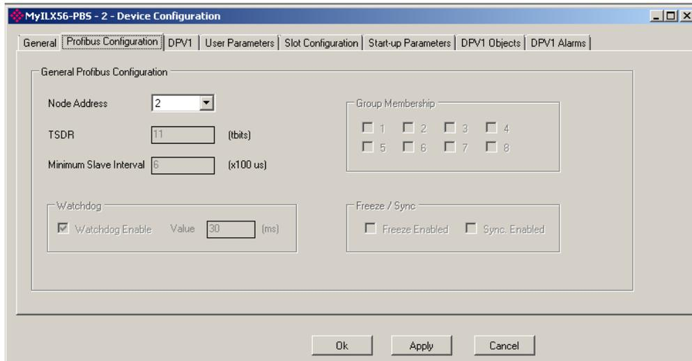
Figure 8.8 –PROFIBUS configuration
