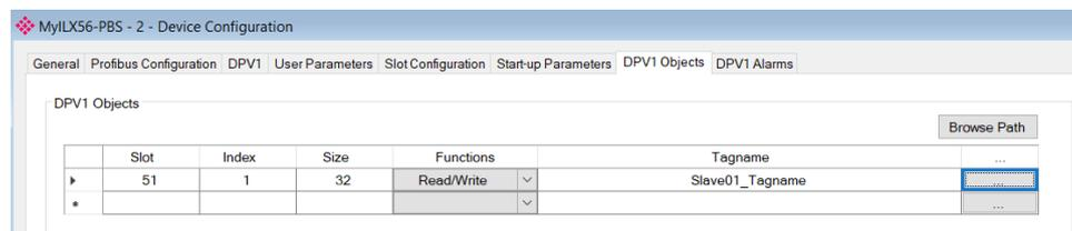
Figure 3.22 – Device DPV1 Objects configuration parameters – Logix
