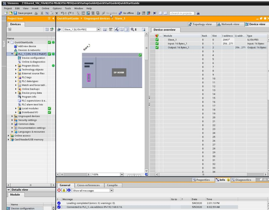
Figure 8.33 – Going online with the Siemens processor
