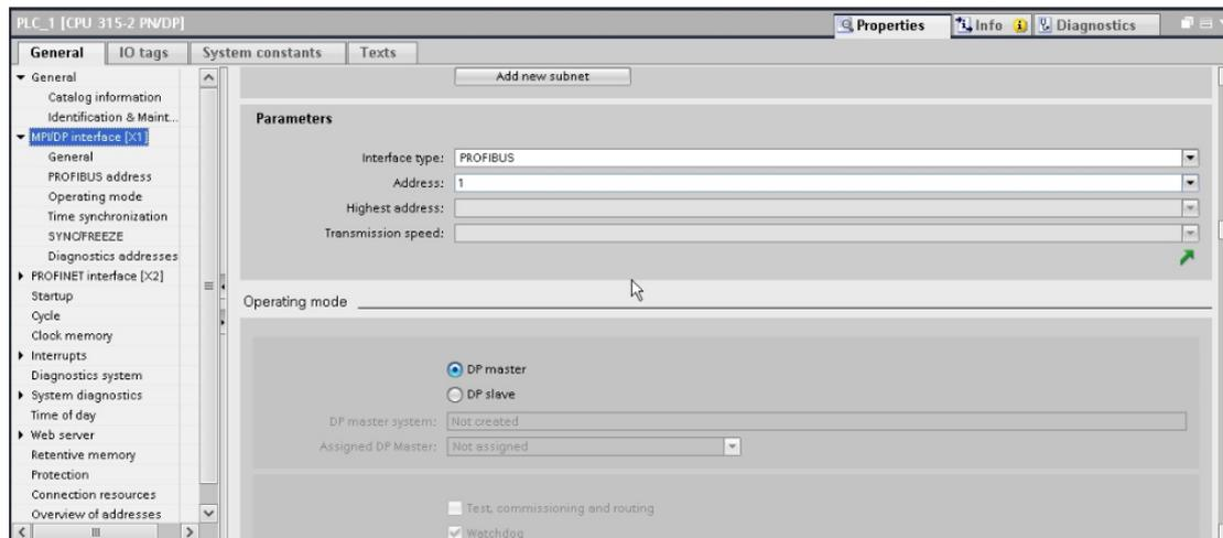
Figure 8.23 – Configuring the MP/DP interface
