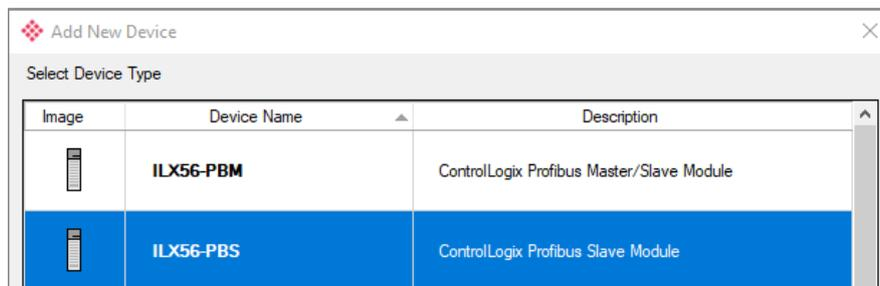
Figure 8.4 – Adding a new ILX56-PBS device
