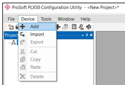
Figure 3.3 - Adding a new device
