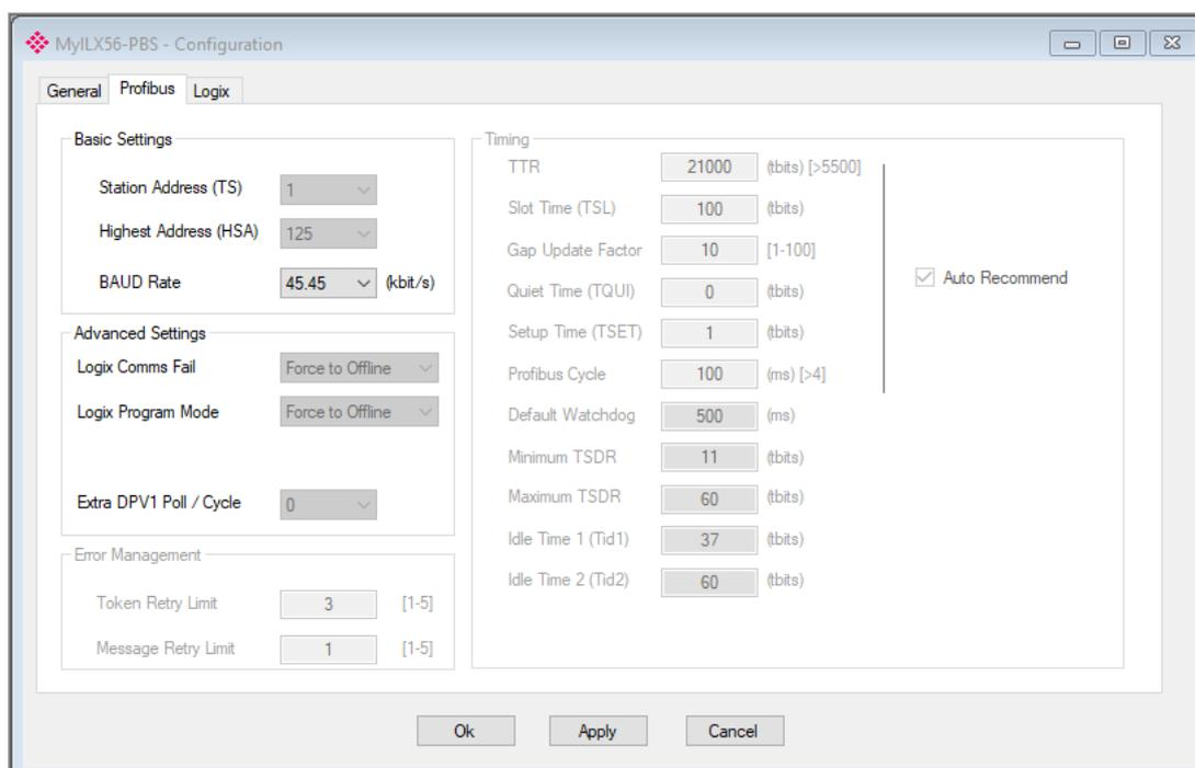
Figure 3.7 – ILX56-PBS PROFIBUS configuration – Slave Mode
