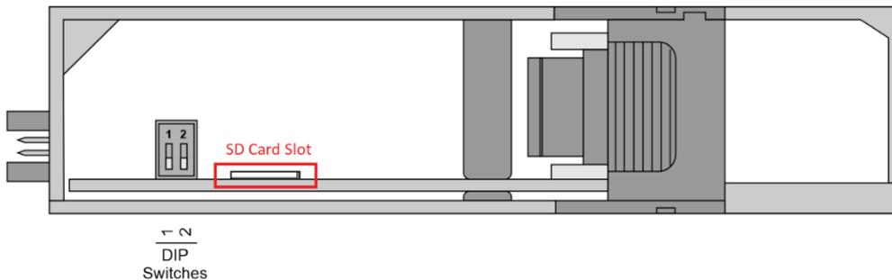
Figure 3.44 – Module Bottom View – SD Card Slot
