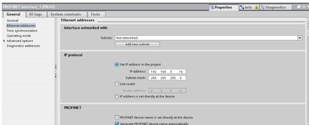
Figure 8.22 – Configuring the device's IP address
