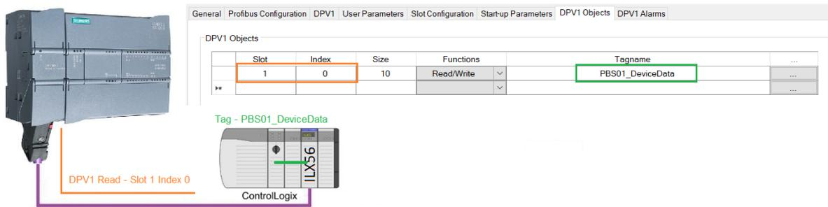
Figure 4.4 – ILX56-PBS DPV1 Object exchange
