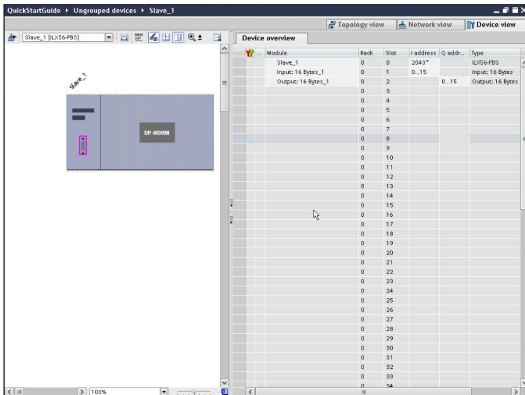
Figure 8.27 – Changing the I address and Q address
