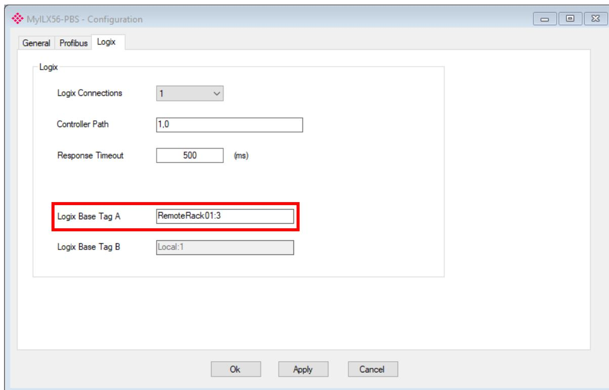
Figure 3.36 – Logix Base tag assignment in PLX50CU
