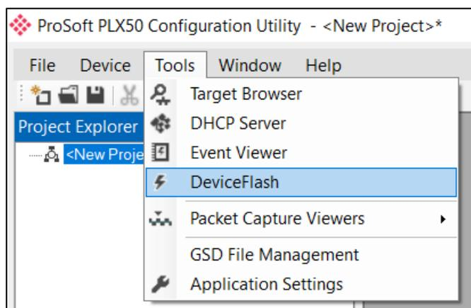
Figure 4.8 - DeviceFlash Tool
