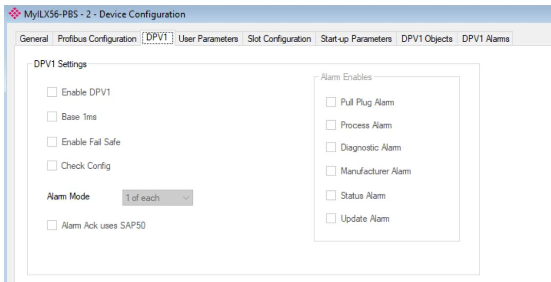
Figure 3.16 – Device DPV1 configuration parameters (legacy device)
