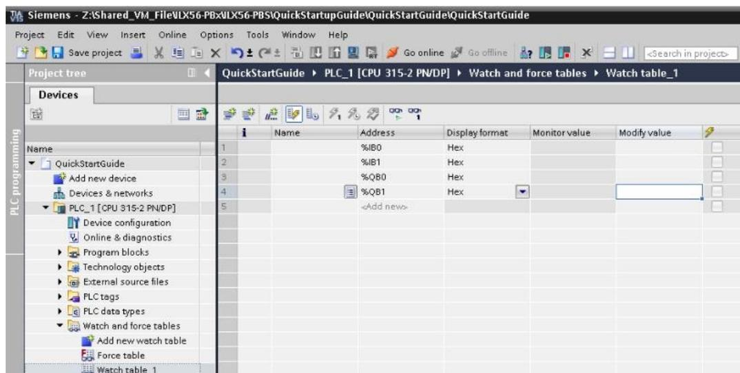
Figure 8.28 – Changing the I address and Q address
