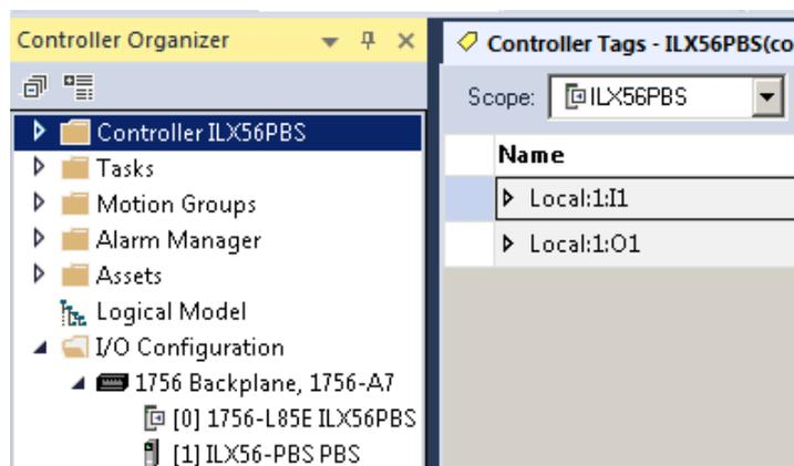
Figure 3.35 – Logix Base tag assignment in Studio 5000
