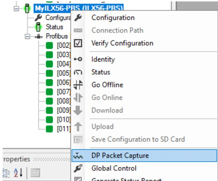
Figure 5.9 - Selecting PROFIBUS Packet Capture
