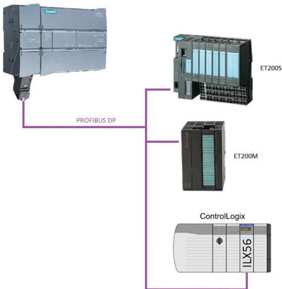
Figure 1.1 – Typical ILX56-PBS PROFIBUS Slave architecture
