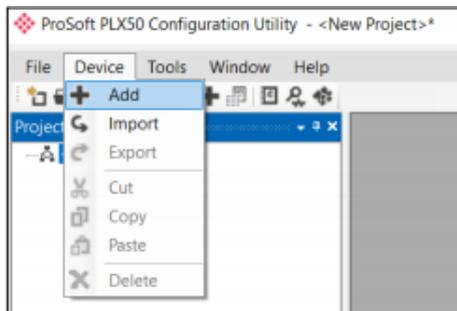
Figure 8.3 – Adding a new device
