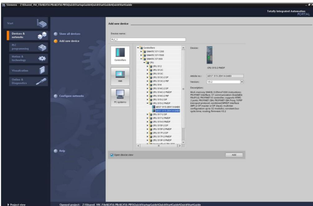
Figure 8.20 – Adding the processor as a new device
