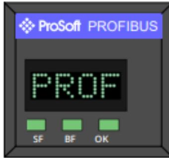
Figure 5.1 - ILX56-PBS LEDs
