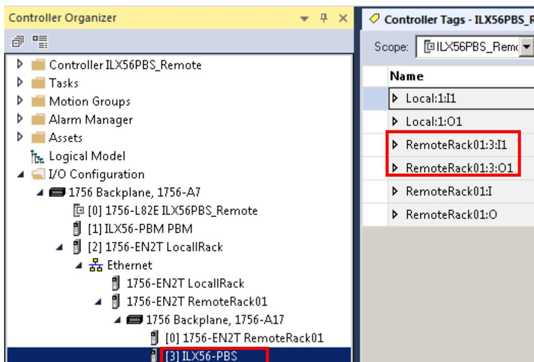
Figure 3.37 – Logix Base tag assignment in Studio 5000
