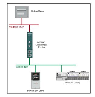
Figure 2 - Typical setup for Modbus TCP/IP server to ControlNet I/O
