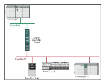
Figure 3 - Typical setup for ControlNet Target to EtherNet/IP I/O
