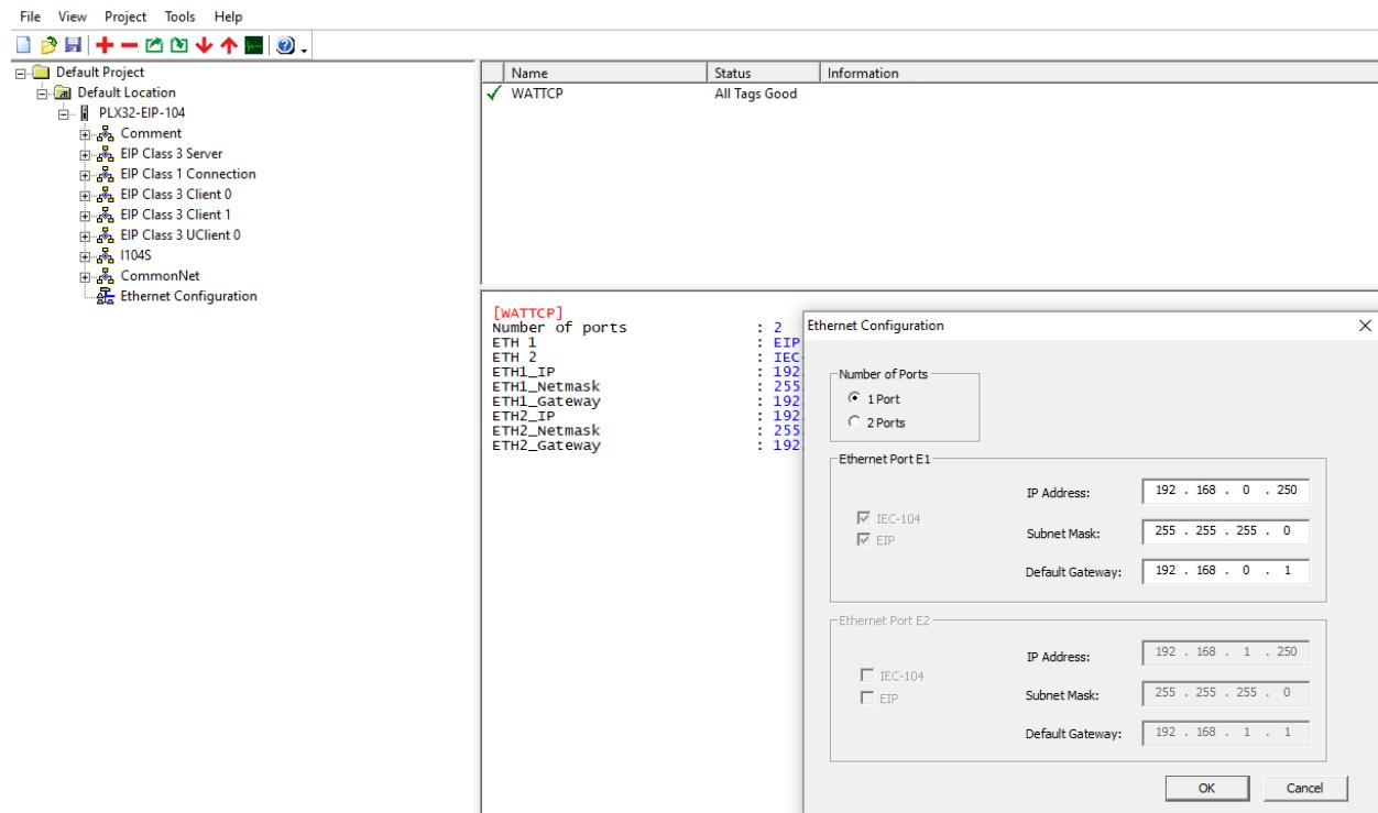
The PLX32-EIP-104 module uses this IP address for downloading of the configuration file and diagnostics as well as communication with Ethernet devices. The default IP address of the module is the 192.168.0.250 as shown above.
