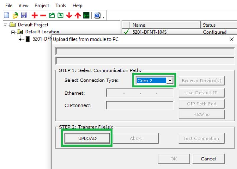
This will upload the configuration from the 5201-DFNT-104S module. Now would be a good time to “Save” the PCB file (or .ppf file).
