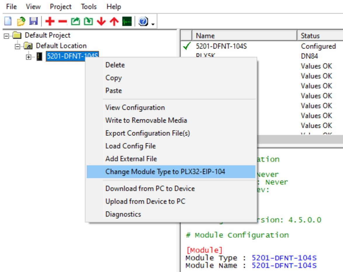
This will automatically convert the configuration file to the PLX32-EIP-104.
