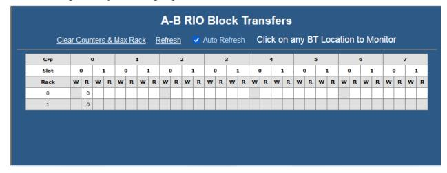
Any cell in the table with a number indicates a location where a block transfer has been defined on an active or monitored rack. The numbers are counters, from 0-63, that indicate how many times the block transfer has been updated. The counters wrap around to 0 after they reach 63.
