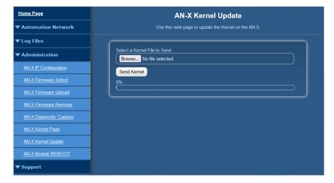
AN-X displays a progress bas as the file is transferred. When the transfer is complete, the AN-X still has to copy the kernel file to the microSD card. When the file copy is complete, the AN-X displays a message to indicate that the file was copied successfully. Stay on this web page until AN-X indicates that the file has been written to the microSD card, then click the REBOOT button to restart the AN-X.
