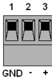
Maximum power consumption is 3.6 watts, 300 mA @ 12VDC, 150 mA @ 24VDC.
