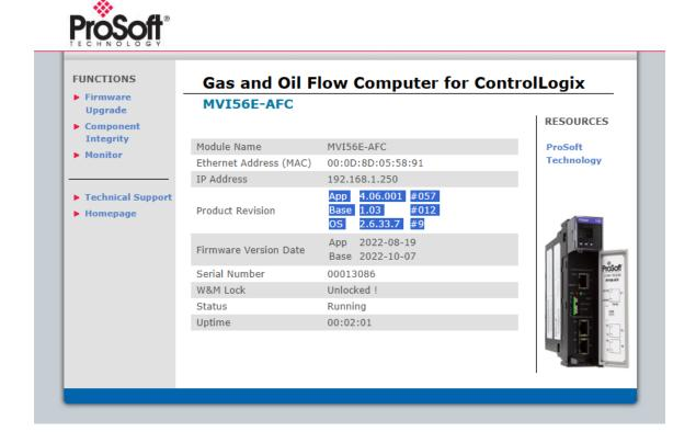
**Note:** Downgrading the application image performs an application cold start / reset to factory defaults. Changing the application image removes the application image. Remove if the module does not correctly operate, and downgrade to the last working application image.
