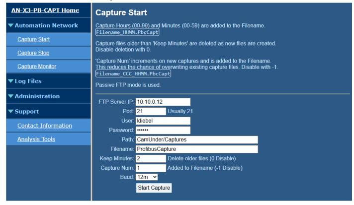
This page is used to specify Profibus, FTP and other parameters, as well as to start a capture.
