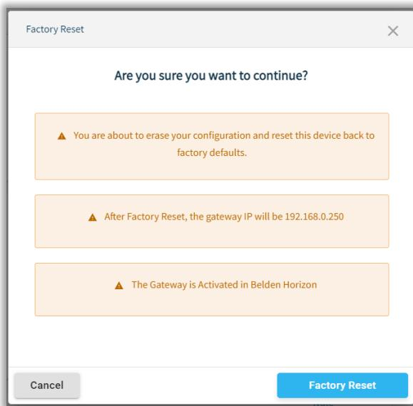
**5** Click **FACTORY RESET** to initiate the factory reset procedure.
