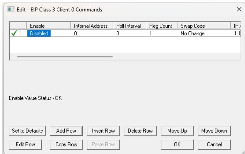
5 Edit the parameter values for the CIP data table command. The example below will configure the ELX-EIP-MBTCP container to write **10** integer values (stored at *Internal Addresses 0 to 9*) to the server IP **192.168.0.30** (controller tags *DestinationTag[0]* through *DestinationTag[9]*). The command will continuously be sent every second.
