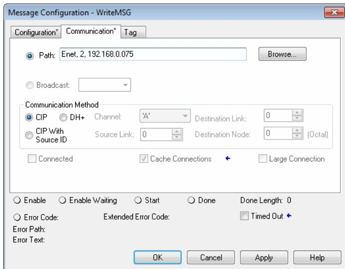
4 Select **CIP** as the **COMMUNICATION METHOD**. The **PATH** specifies the message route from the processor to the container. Path elements are separated by commas. In the example path shown:
