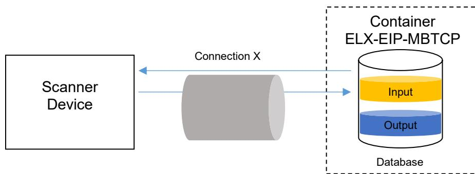
By default, the ELX-EIP-MBTCP container is configured with specific internal I/O memory locations that map to the PLC's Input Image (data received from the PLC) and Output Image (data sent to the PLC) for each connection.
