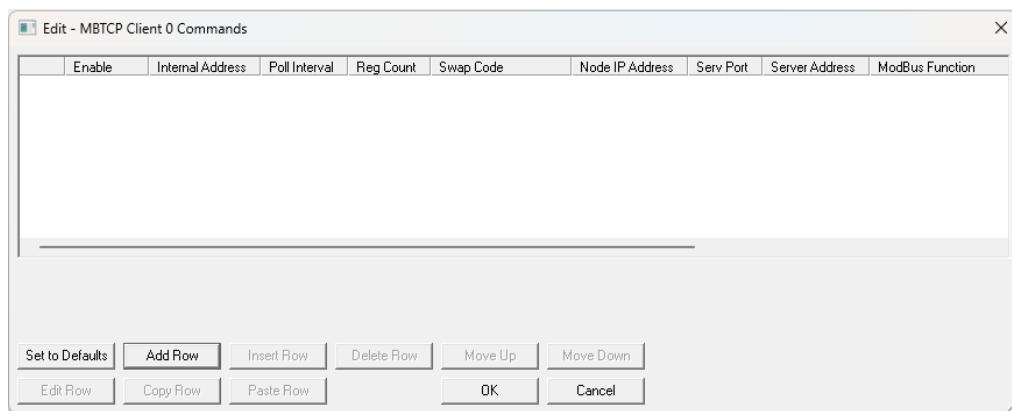
4 The example below configures the ELX-EIP-MBTCP container Modbus Client to write **10** holding register values stored at container database addresses **0** to **9** to the Modbus TCP server IP **192.168.0.30** starting at address 40101. The command will be sent continuously every second.
