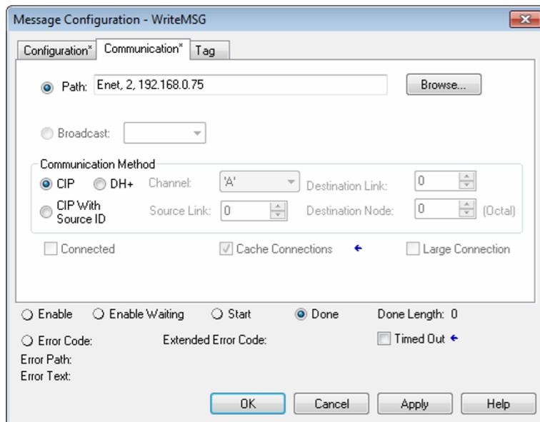
4 Select **CIP** as the *Communication Method*. The *Path* specifies the message route from the processor to the EIP driver. Path elements are separated by commas. In the example path shown:
