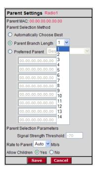
With **Parent Branch Length**, the IH will choose its parent strictly by the number of repeaters between it and the Master radio. If Branch Length of 1 is chosen, the IH will link only to the Master radio. If Branch Length of 2 is chosen, the IH will link only to an IH that is linked to the Master radio, and so on.
