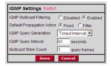
RLXIB-IHW radios support IGMP v1 and v2. The default operation of the RLXIB-IHW radios is to have IGMP functionality enabled, although the user can disable IGMP entirely. Additionally, the user can specify settings associated with IGMP filtering and snooping. Unknown multicast addresses can be sent to all ports (flood) or to none (filtered) by changing the IGMP Multicast Filtering option. The user can specify whether the radio will generate IGMP queries, and configure the query interval time.
