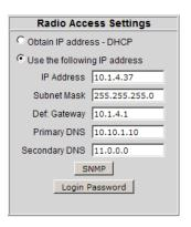
If a DHCP (Dynamic Host Control Protocol) server is configured on your local area network, the DHCP server can assign IP addresses automatically. If you prefer to assign a Static (Fixed) IP address, select **USE THE FOLLOWING IP ADDRESS**, and then enter the IP Address, Subnet Mask and Default Gateway in the Radio Access Settings area of the IH Radio web configuration form.
