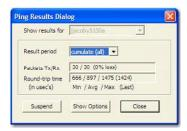
This dialog box displays statistics on the minimum, maximum and average latency between two points on the network.
