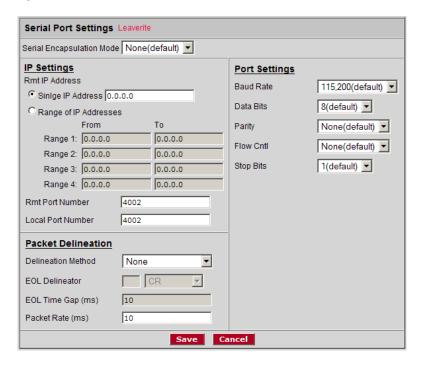
Use this page to configure the way serial data packets are encapsulated and transmitted over an Ethernet network.
