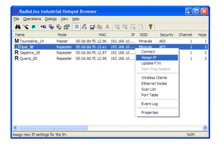
Connect (page 72): Log in to the Radio Configuration / Diagnostic Utility to configure a radio or check diagnostics.
