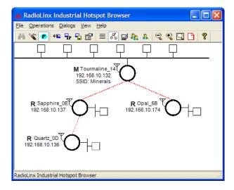
The Topology view shows a diagram of the network's wireless connections. Use this view to see whether all the radios are linked, and that you approve of the way the radios are linked. A radio that is not linked to a parent will show as a circle outlined by a flashing dashed red line. It may be near the bottom of the window, so scroll down to view all available radios. To change how radios link to the network, see Parent Link settings (page 48).
