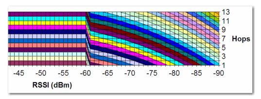
Once per second, the RLXIB-IHW radio evaluates the link it has to its parent to determine if this link is the best parent to use. A cost is calculated for each entry and can be seen in the column labeled "Cost" in the preceding table. The cost calculation is based not only on the strongest signal, but on several other factors to provide optimum network communication.
