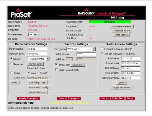
To configure a Master radio, make the following changes to the web configuration form:
