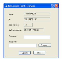
In order for your RadioLinx Industrial Hotspot radio to communicate with other RLXIB-IHW devices, all radios on the network must use the same firmware version.
