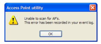
This error occurs when the IH Browser attempts to scan for radios and no valid network connection exists on the PC, wired or wireless.
