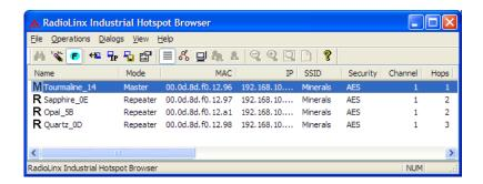
List View shows a list of all the connected radios in a grid, arranged similarly to data in a spreadsheet. Resize the window or scroll across to see all of the available columns. Click between column headers and drag to the left or right to resize columns. Click on column headers and drag to the left or right to re-order columns.
