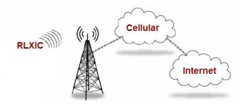
The RLXIC-EH will perform a **one-to-one** routing for all internet traffic to and from the computer or other end device. One-to-one means that your RLXIC-EH will provide a connection for one device to the Internet at a time. In Private Mode, the RLXIC-EH will provide NAT (Network Address Translation) for the computer or other end device.
