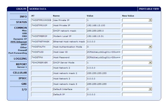
Using a private IP insulates the PPP client from changes in IP addresses of the underlying network. The will perform basic NAT-like address translation on all packets.
