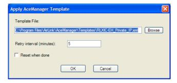
4 Set the Retry Interval and check if you want to have the modems Reset when the template has been applied.
