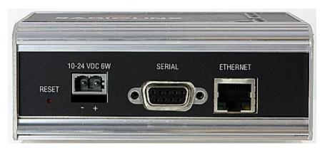
From left to right: Power connector, Serial port, and Ethernet port. Use the Ethernet cable to configure the radio for the first time.
