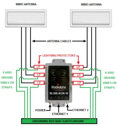
Ground wires or straps must be tied from each active lightning protector to a secured earth ground. (LP Grounding Wires must be 6 AWG, or larger.)
