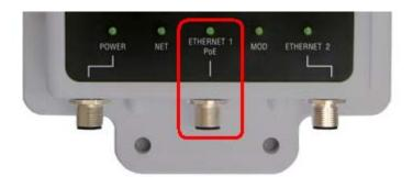
From left to right: Power, Ethernet 1, and Ethernet 2 Use the Ethernet cable to configure the radio for the first time.
